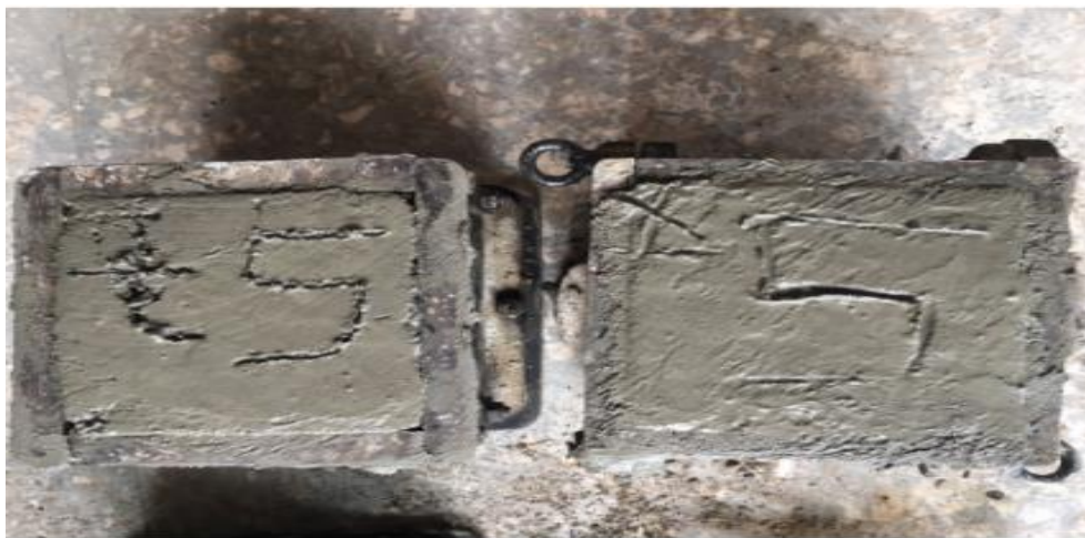
Figure 4: Fresh concrete cubes
